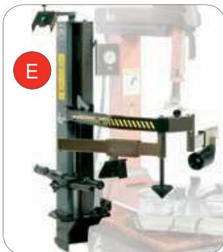
**(EN) UNIVERSAL PNEUMATIC DEVICE UPH & BPS (OPTIONAL):** Universal auxiliary device UPH & BPS, which assists the operator to easily mount and demount particularly tough or low profile tyres such as «Run-Flat». This patented system allows to handle the second tyre bead without using the lever, thus avoiding any risk of rim damaging. Other right side help arms (SPH or TPH) are also available on demand.
