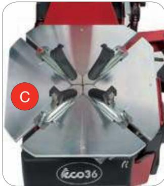
**(EN) SELF-CENTERING TURNTABLE:** System able to lock rims from 10" to 25" without adapters and adjustments: internal clamping capacity 10"-22", external 13"-25". It employs unique rod geometry to ensure constant and even clamping power throughout all rim diameters.
